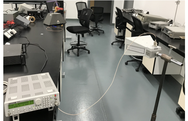
Fig. 4. 2-Antenna method Radiation Pattern Setup.
